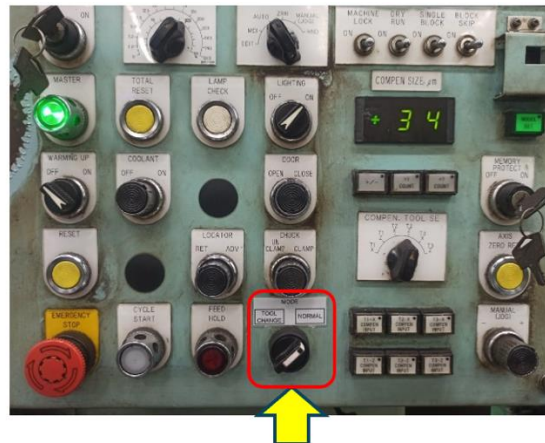
Figure 8. Addition of mode selector for tool change
