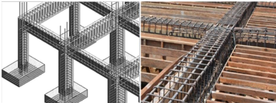
Figure 1. Beams with vertical stirrups
