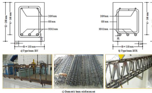
Figure 4. Detail of concrete beams
