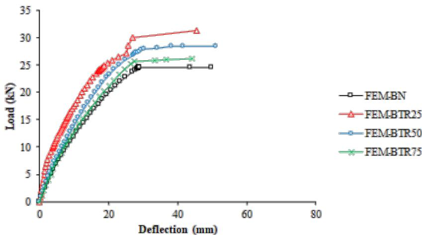
Figure 8. Load-deflection of the FEM results
