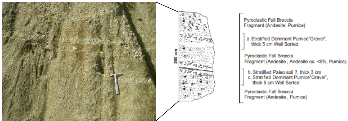
Figure 13. The figure shows a pyroclastic fall profile at the site of the Tirta Husada hot spring and mud pool.
