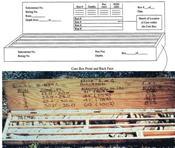
Figure 2. Box Marked Core
