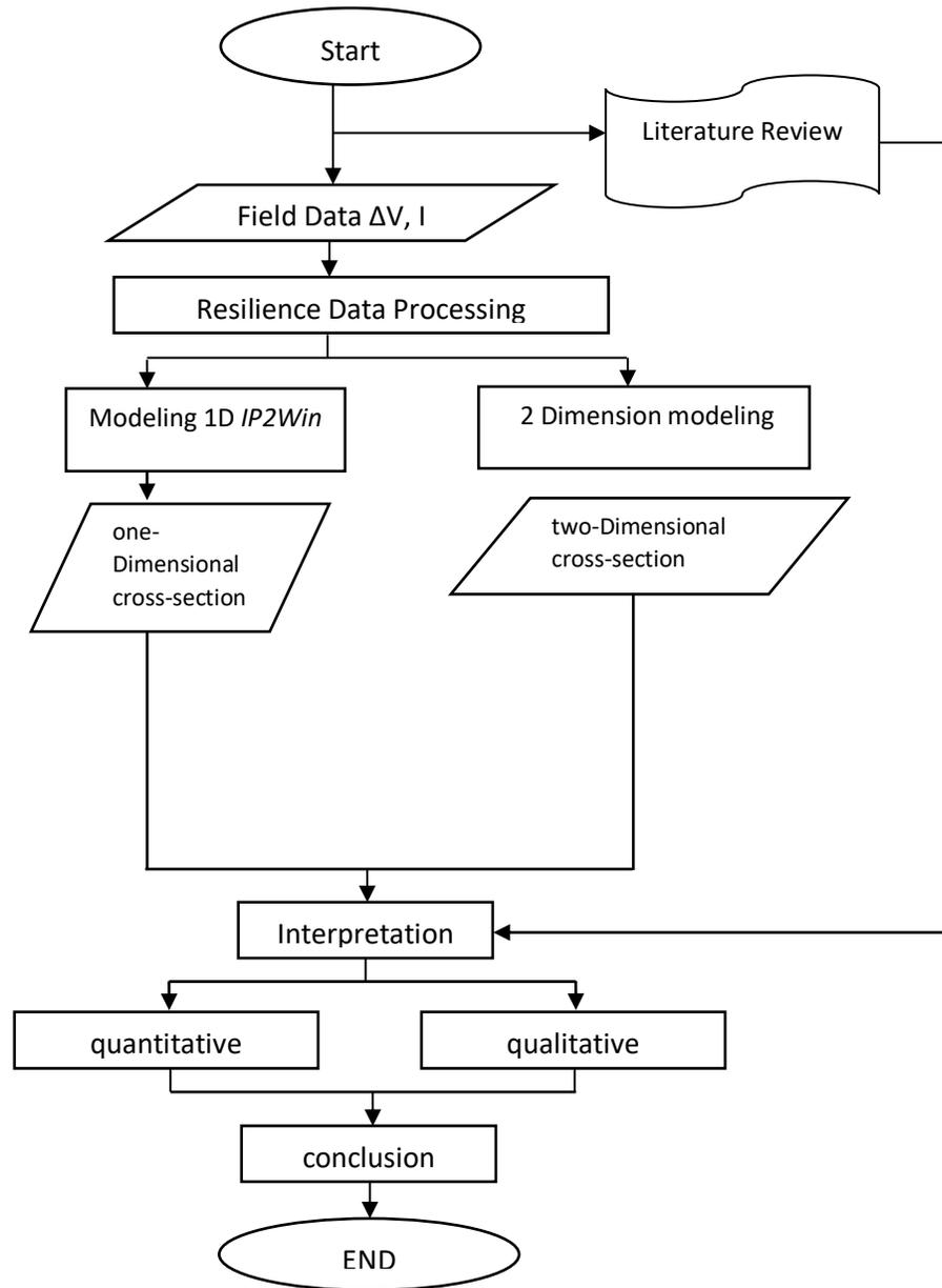
Figure 7. Data Processing Flowchart
