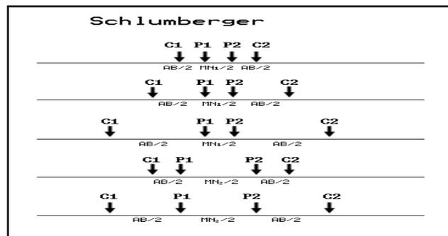
Figure 3. Electrode Displacement of the Schlumberger Configuration
