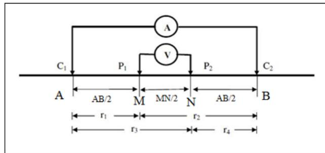
Figure 2. Electrode Arrangement of the Schlumberger Configuration
