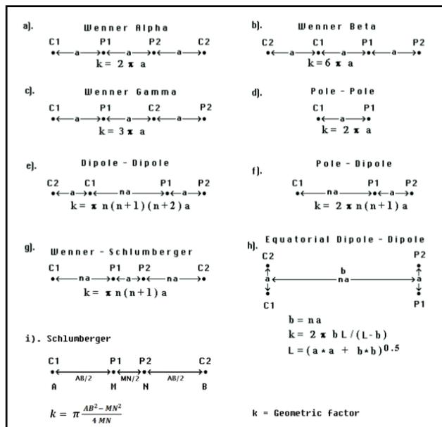
Figure 1. Electrode Configuration used in resistivity measurement and Geometry Factors (Modified Loke, 1999)
