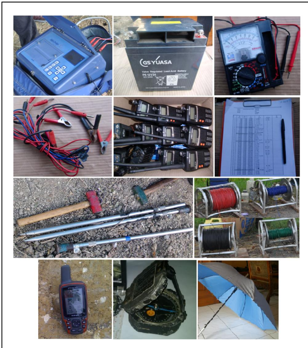
Figure 5. Geoelectrical measuring equipment
