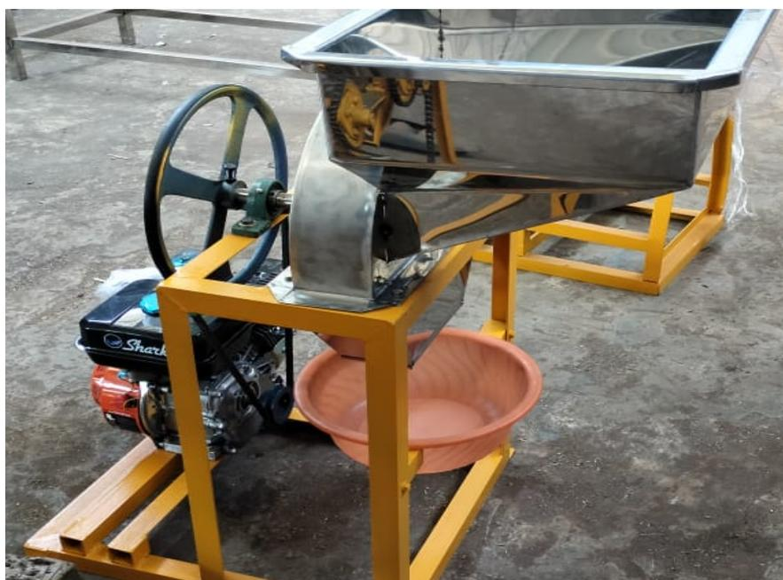
Figure 2, The empon-empon chopper machine
