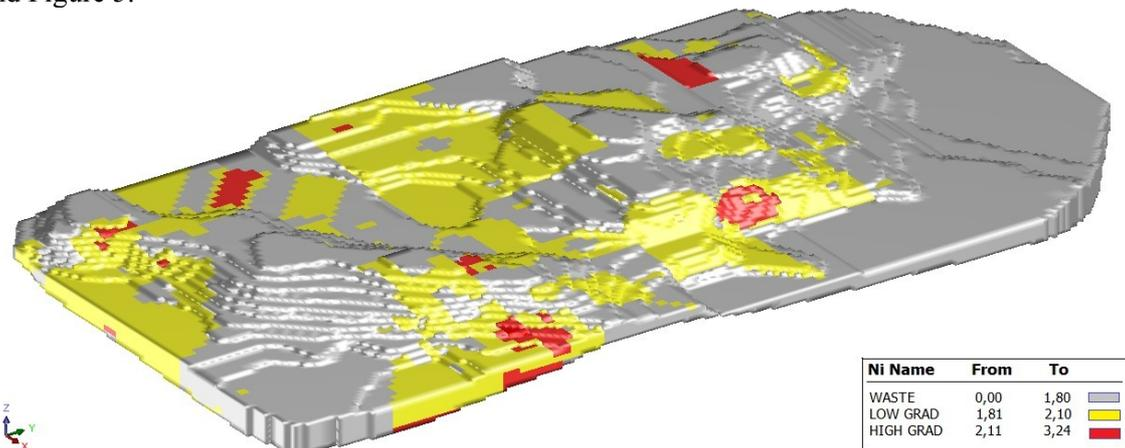
Figure 4. Geological 3D model of the nickel deposit
