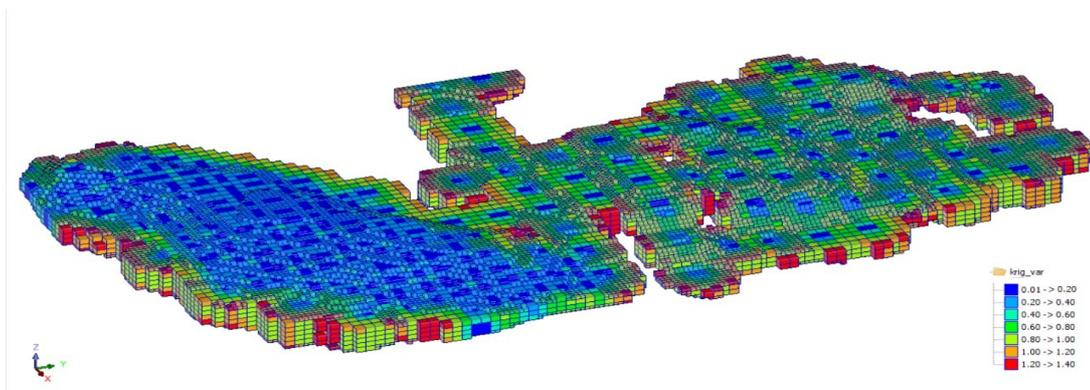
Figure 9. The kriging variance showing the sample configuration index
