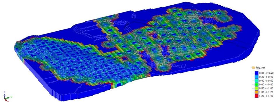
Figure 8. 3D block model showing the distribution of nickel grades.
