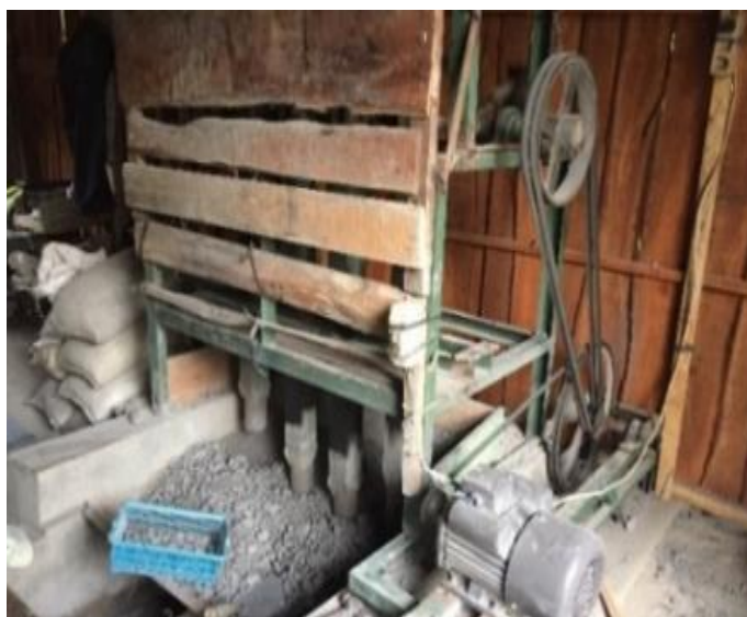
Figure 1. Gold Processing in Pancurendang Village Using Pound, Gelundung, and Mercury Tools (Muryani, Hudawan, & Rahmah, 2020)
