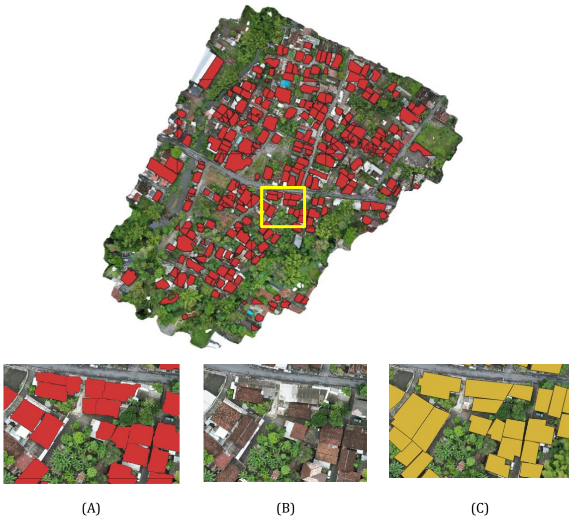
Figure 6. Example of Well-Detected Building Locations (A) Segmentation, (B) Orthophoto, (C) Ground Truth
