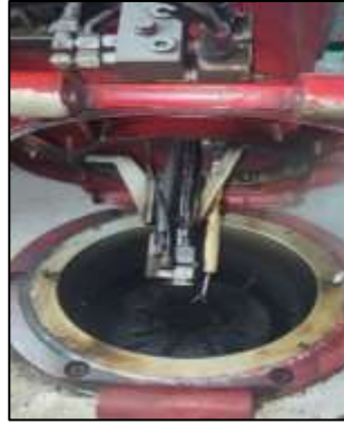
Figure 5. Cleaning and adjusting space between electrode
