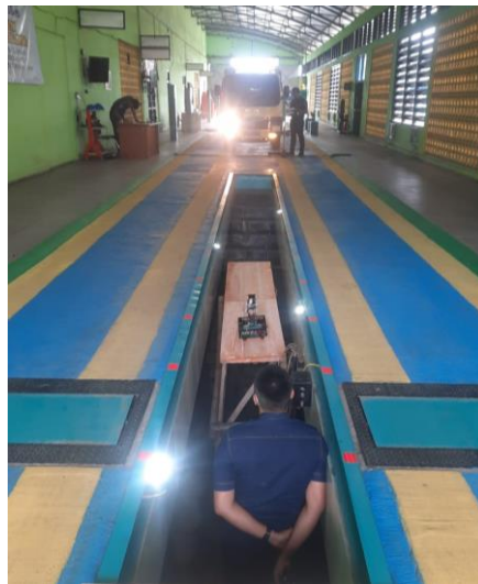
Figure 12. Inspection process lower vehicle
