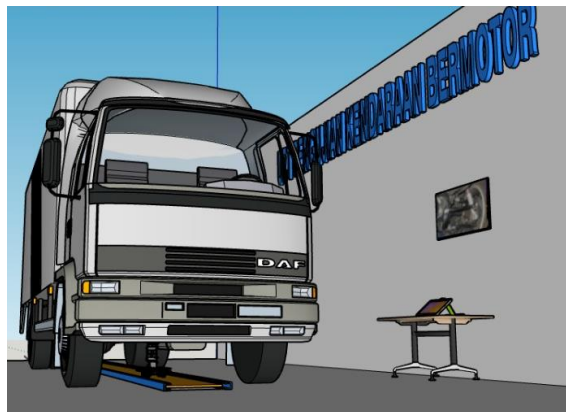
Figure 7. Illustration testing inspection lower vehicle-based robotics
