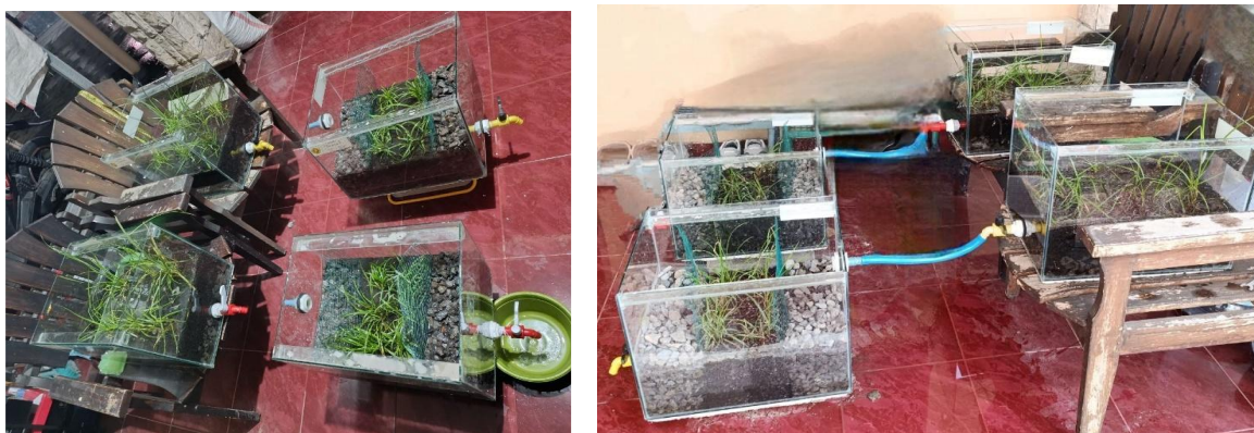
Figure 3. Constructed Wetland Experiment
