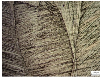
Figure 2. Microstructure of a shape memory alloy with a needle-like shape
